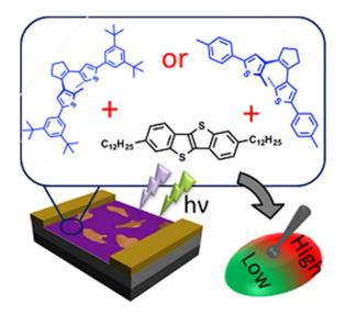
Schematic illustration of the field-effect transistor based on blends of photochromic molecules bearing different alkyl substituents (shown in blue) blended with a small molecule organic semiconductor (shown in red). This blend results in high or low performance switch under illumination depending on the photochromic molecule.
